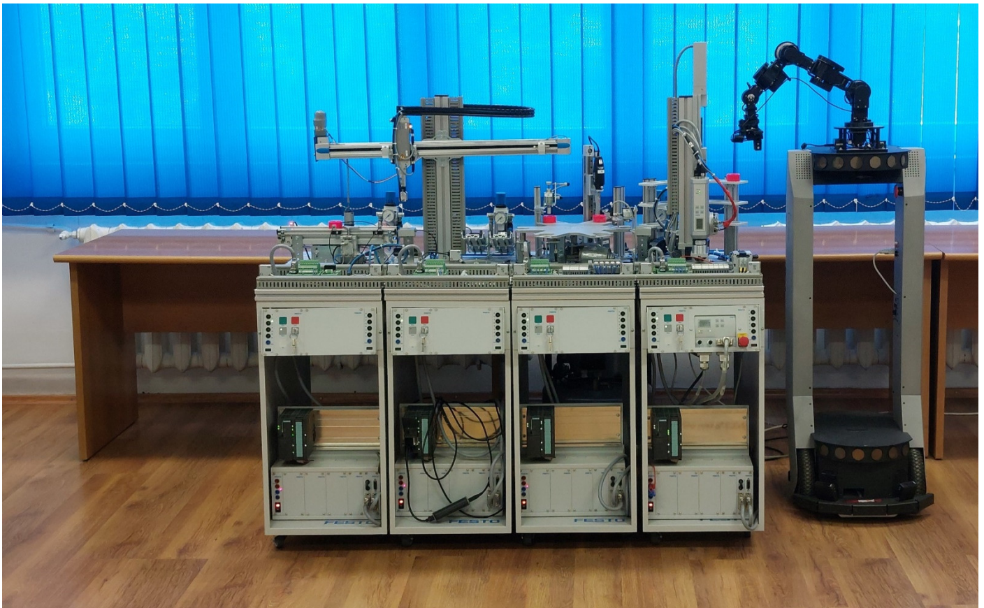
Figure 1. Festo MPS 200 assisted by CAS (ARS PeopleBot equipped with RM Cyton 1500 and MVS).
