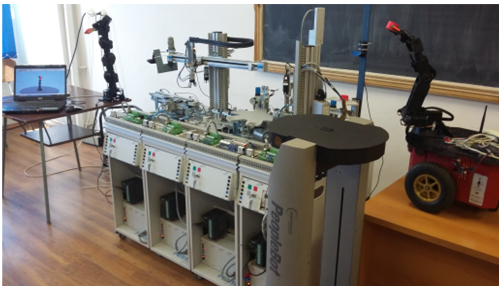
Figure 1. Processing/reprocessing mechatronics line (P/RML) assisted by autonomous robotic systems (ARSs), robotic manipulators (RMs) and visual servoing systems (VSSs).
