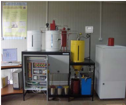
Fig. 2. The biological wastewater treatment pilot plant, from “Dunarea de Jos” University of Galati.
